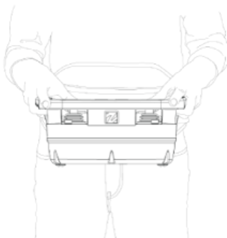
Fig. 1 Working position with a Tele Radio transmitter while using the Tele Radio waist belt
