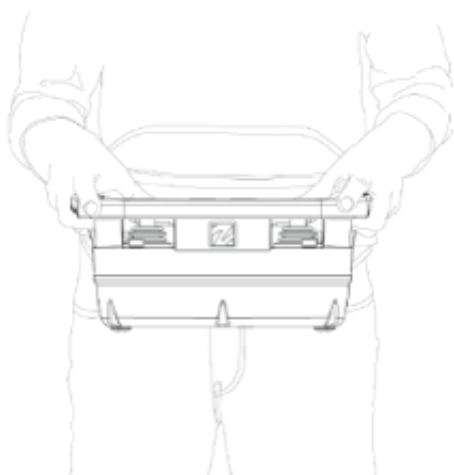
Fig. 1 Working position with a Tele Radio AB transmitter while using the Tele Radio AB waist belt
